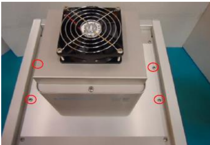
Figure 10. Remove ECE Reflector Assembly
